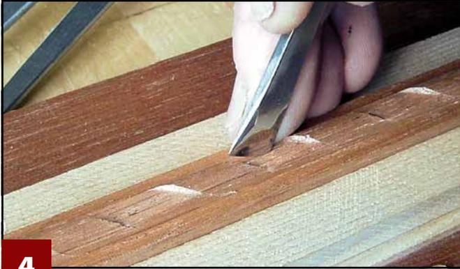
**4** **Make these cuts the length of the molding.** Remember, the deepest point of the cut is in the middle of the length of the stick, where you have plunged the corner of the blade down. Your goal is to get an even sense of the line of the stick passing from flat to flat by making controlled, matching cuts on both sides of the stick. It is important to keep the depth of the cuts consistent from one flat to the next.
