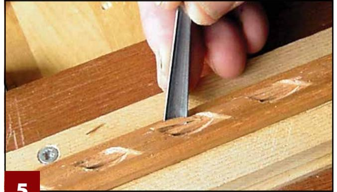
**5** **Remove the chip of wood on either side of the stick.** Make a scoop cut with the corner of an 8mm #3 fishtail gouge. As you make this cut, bring the handle back towards you so the other gouge corner arcs down to meet the stab cut alongside the stick. This cut releases a chip of wood shaped like an orange segment. Work all along one side; then work back along the other side. When you have finished both sides, the stick will be clearly visible.
