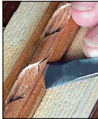
**6** **Shape the sides of the ribbon.** Use an 8mm #3 fishtail gouge to make two vertical stab cuts from the edge of the stick to the quirk to define the edge of the ribbon. Work along one side from end to end, and then work on the other side. Keep the line of the ribbon edge flowing. Slide a 14mm #1 fishtail chisel along the quirk to free the chip, similar to the chip you removed when carving the pea molding.
