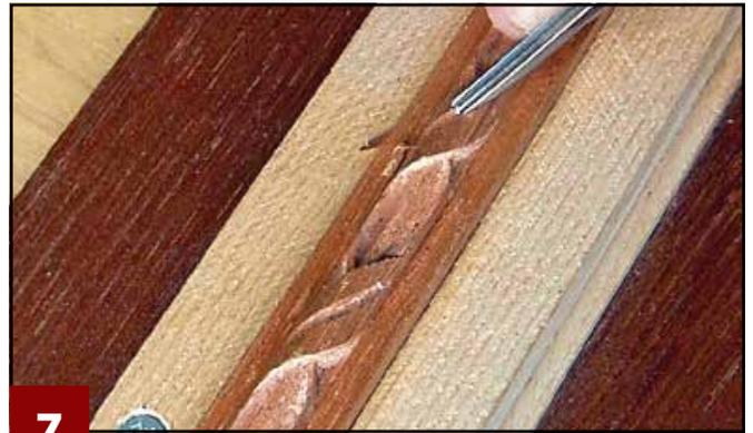
**7** **Add the final ribbon detail.** Run a little groove with a 2mm #11 gouge along the center line of each section of ribbon. It should be heavier in the middle, fading away as it winds around to the quirk. This line not only adds a little flair to the molding, but it also helps the viewer see the winding nature of the ribbon. A similar embellishment would serve the same purpose if added to the rope molding.
