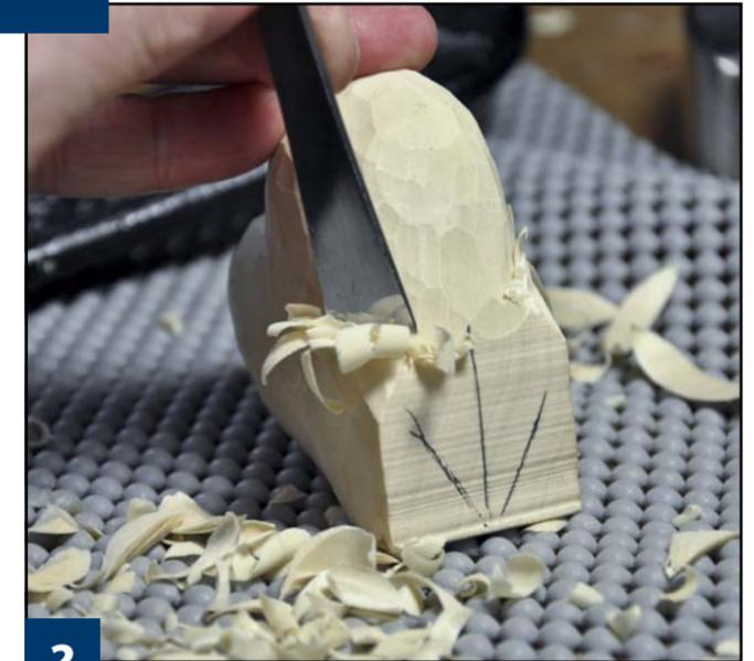
**2 Carve the hearts.** Cut the perimeter of the hearts and draw a centerline along the edges. Place the heart on a non-skid mat, clamp the bottom to the bench, and use a  $\frac{3}{4}$ " (or 20mm) #3 fishtail gouge to round the top. Refine the line between the two halves with a  $\frac{1}{4}$ " (6mm) 45° V-tool. Repeat the process on both sides. Then, brace the heart on a non-skid pad and round the bottom of the heart.
