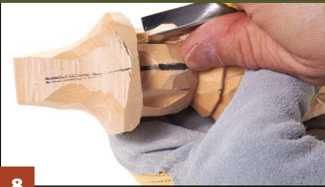
8 Shape the outside of the face. Mark the width of the face (the hairline) and use a V-gouge to carve the hair back so the face protrudes. Clean up the cuts with a knife. Repeat the process on the other side of the face, and match the depth of the cuts.
