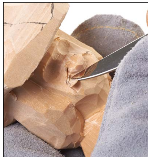
11 Refine the nose. Use the knife to make a stop cut around the wings of the nose, and then carve up to the stop cut to separate the wings from the cheeks. Round the tip of the nose slightly. Make a stop cut around the outside of the nostril with the tip of the knife, and then carve up to the stop cut to remove a chip. Draw the smile lines, make stop cuts on the lines, and carve up to these stop cuts to define the smile lines and start shaping the dental mound.
