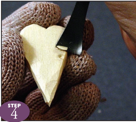
STEP 4 Use a #3 5/8" gouge to carve away and contour the face of the heart as shown.
