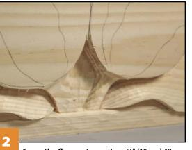
Carve the flower stems. Use a  $\frac{3}{8}$ " (10mm) #9 gouge to separate the stem from the tulip. Do not use a V-tool. Drop the stems down to about  $\frac{1}{8}$ " (3mm) above the leaf. Round the sides of the stems with a  $\frac{7}{16}$ " (12mm) #5 gouge.
