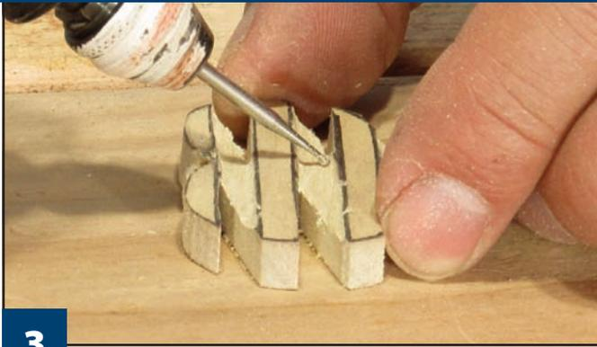
**3** **Begin carving the pendant.** Carve away about  $\frac{1}{16}$ " (2mm) of wood from the shaded areas on the front and back of the pendant. I use a  $\frac{1}{16}$ " (2mm)-diameter ball-shaped engraving bit. Work slowly to keep from nicking the sides. The goal is to keep the surface as smooth as possible.
