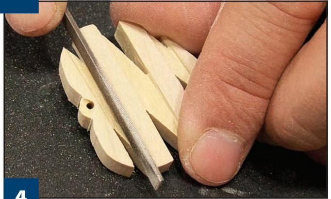
**4** **Smooth the carved areas.** Use a flat needle file to smooth the recessed areas of the pendant. When you're finished, you should have raised flat surfaces and recessed flat surfaces. It is easy to break the pendant when using the files. Support the back of the piece and use light pressure on the file.
