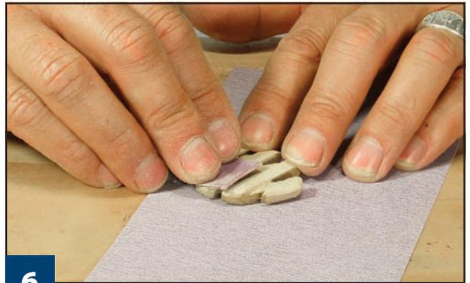
**6** **Sand the pendant.** Use a small piece of fine-grit sandpaper to smooth the surface of the pendant. A well-sanded surface will help ensure a smooth finish.
