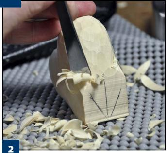
Carve the hearts. Cut the perimeter of the hearts and draw a centerline along the edges. Place the heart on a non-skid mat, clamp the bottom to the bench, and use a 34" (or 20mm) #3 fishtail gouge to round the top. Refine the line between the two halves with a 1/4" (6mm) 45° V-tool. Repeat the process on both sides. Then, brace the heart on a non-skid pad and round the bottom of the heart.
