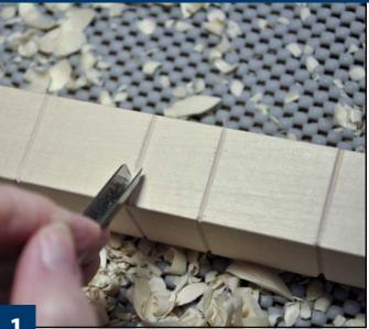
repare the letter board. Cut the board to size and sand it smooth. Figure out what you want to say, and then mark in 11/2" (38mm)-wide blocks for letters and 15/16" (24mm)-wide blocks for the spaces between letters. Carve along each of the lines with a 1/4" (6mm) 45° V-tool to separate each of the blocks.
