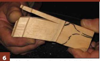
**End the splits.** Continue splitting the feather block until the cuts align with the back of the head, ¼" to ¾6" (6mm to 8mm) from the edge of the block. You will discard the un-split piece later.
