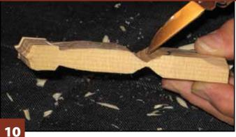
**Remove the shoulder.** Bevel the shoulder down to the hinge, taking care not to thin the hinge any farther or to leave any shoulder. There should be no step on the hinge area, just a perfect V shape.
